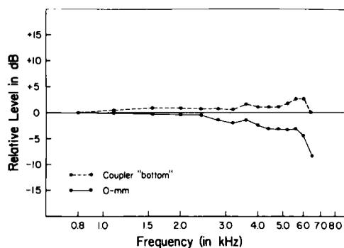
Fig. 2. Pressure levels measured at the 0-mm and coupler bottom probe positions plotted in relation to the levels observed at the 5-mm probe position in a Zwislocki coupler.
