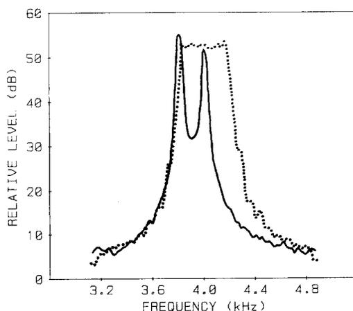
FIGURE 1. Long-term RMS spectra of the two types of warble tones. The nominal frequency of both stimuli was 4000 Hz. The solid line illustrates the spectrum of the FM stimulus produced by the Saico SC8 audiometer. The dotted line illustrates the spectrum of the FM stimulus produced by the Grason-Stadler GSI10 audiometer.
