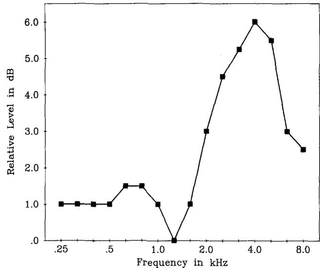
FIGURE 5. Main difference in input to ITE hearing aid microphone and OTE hearing aid microphone when both were exposed to the same broad-band sound field signal. The ITE data are plotted relative to the OTE data.  $N = 10$  independent ears.
