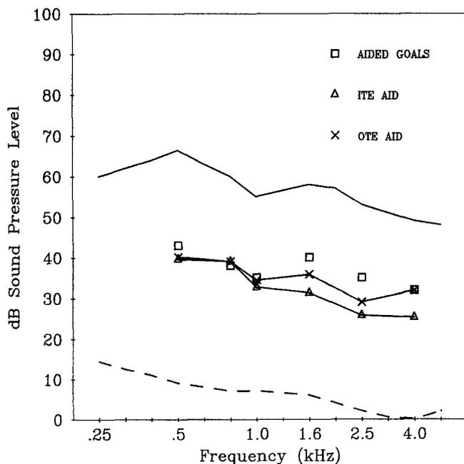
FIGURE 4. Mean aided sound field threshold goals, mean aided sound field thresholds for ITE hearing aids, and mean aided sound field thresholds for OTE hearing aids. The solid line shows the one-third octave levels of a speech signal at 70 dB SPL overall level. The dashed line gives the normal, monaural sound field thresholds for 0-degree azimuth tones.
