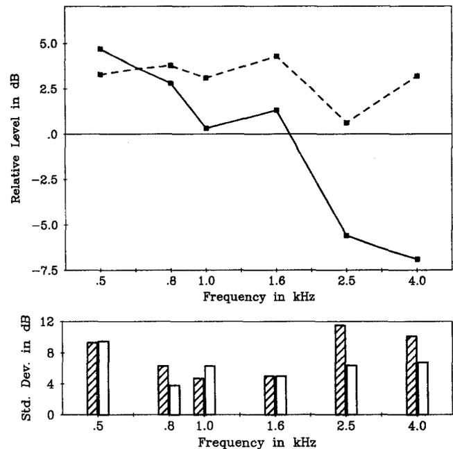
FIGURE 3. Upper panel shows mean functional gain relative to mean coupler gain for ITE hearing aids (dashed line) and OTE hearing aids (solid line). Lower panel gives standard deviations for ITE hearing aids (unshaded bars) and OTE hearing aids (shaded bars).
