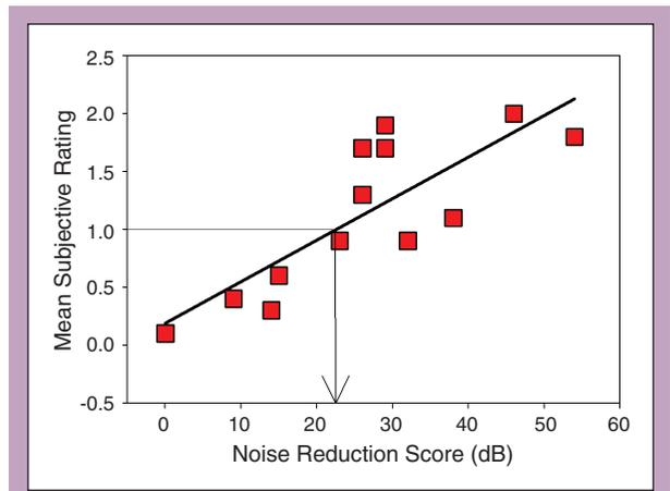
**Figure 8.** Test box Noise Reduction Scores and corresponding mean subjective ratings for 13 hearing aids.
