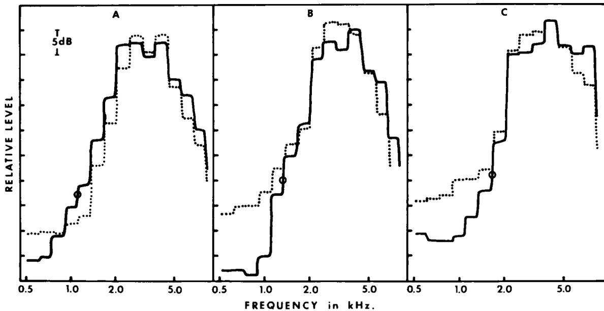
**Figure 3.** Frequency/gain curves, measured in one-third octave band levels, of the two tone control/earmold configurations used with each hearing aid from the third group of instruments. This group was defined as having low cutoff frequencies above 1000 Hz. *Solid lines* depict the electronically modified condition. *Dotted lines* show the acoustically modified condition. *Open circles* indicate the derived low cutoff frequency for each instrument.
