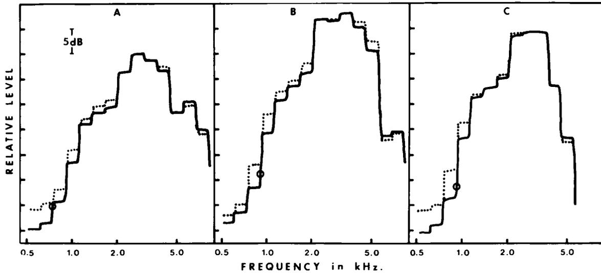
**Figure 2.** Frequency/gain curves, measured in one-third octave band levels, of the two tone control/earmold configurations used with each hearing aid from the second group of instruments. This group was defined as having low cutoff frequencies between 750 Hz and 1000 Hz. *Solid lines* depict the electronically modified condition. *Dotted lines* show the acoustically modified condition. *Open circles* indicate the derived low cutoff frequency for each instrument.
