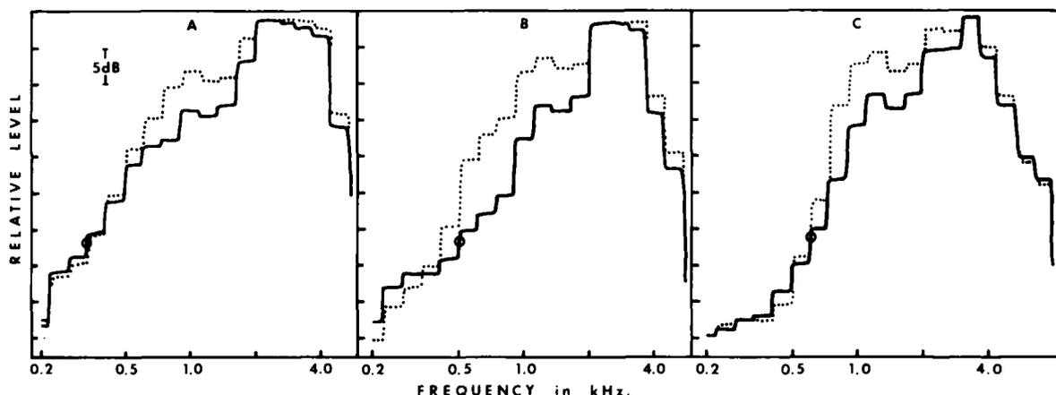
Figure 1. Frequency/gain curves, measured in one-third octave band levels, of the two tone control/earmold configurations used with each hearing aid from the first group of instruments. This group was defined as having low cutoff frequencies below 750 Hz. Solid lines depict the electronically modified condition. Dotted lines show the acoustically modified condition. Open circles indicate the derived low cutoff frequency for each instrument.
