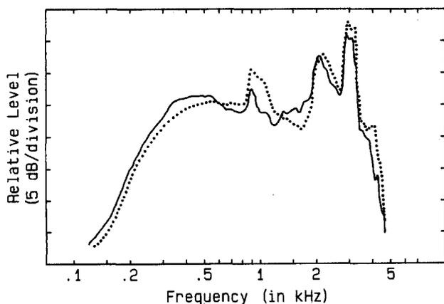
FIGURE 6. Damped (solid line) and undamped (dotted line) preferred listening levels for a typical normal bandwidth, raised speech input level condition. Shown are the Zwislowski coupler frequency responses for one of the three tested hearing aid pairs, averaged across 8 subjects.
