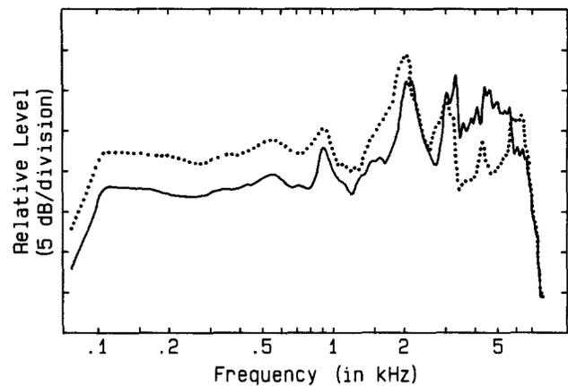
FIGURE 8. Averaged Zwislocki coupler-measured preferred listening levels for the same hearing aid in two different bandwidth conditions. Both conditions employed the same speech level. Dotted line = normal bandwidth; solid line = wide bandwidth.
