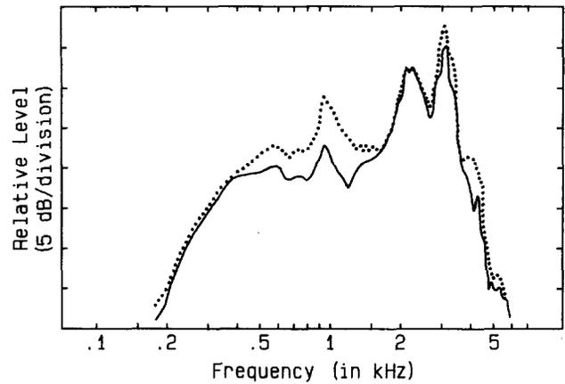
FIGURE 4. Damped (solid line) and undamped (dotted line) preferred listening levels for a typical normal bandwidth, normal speech input level condition. Shown are the Zwislocki coupler frequency responses for one of the three tested hearing aid pairs, averaged across 8 subjects.
