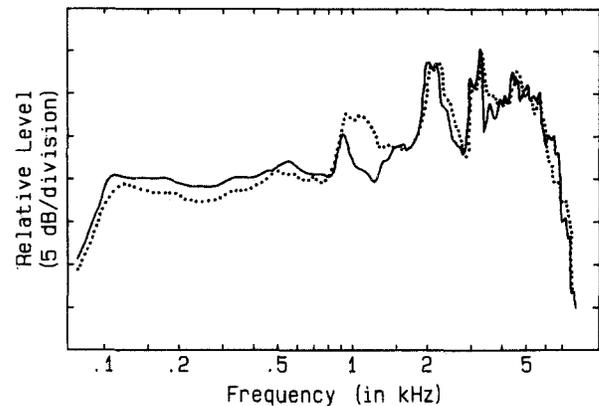
FIGURE 7. Damped (solid line) and undamped (dotted line) preferred listening levels for a typical wide bandwidth, raised speech input level condition. Shown are the Zwislowski coupler frequency responses for one of the three tested hearing aid pairs, averaged across 8 subjects.
