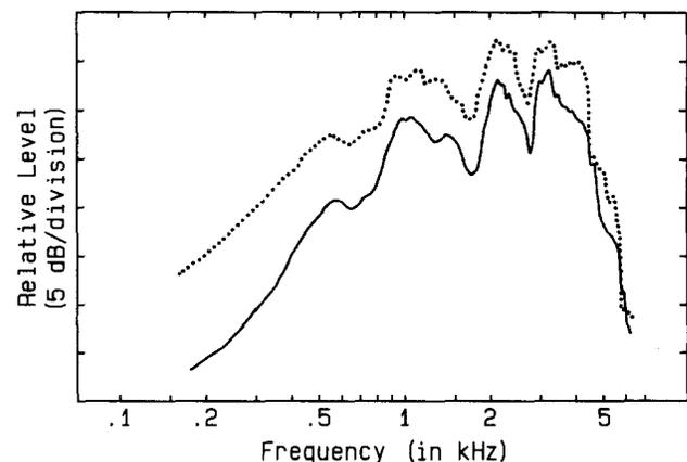
FIGURE 9. Averaged Zwislocki coupler-measured preferred listening levels for the same hearing aid in two different speech input level conditions. Both conditions employed the same bandwidth. Dotted line = raised speech input level; solid line = normal speech input level.
