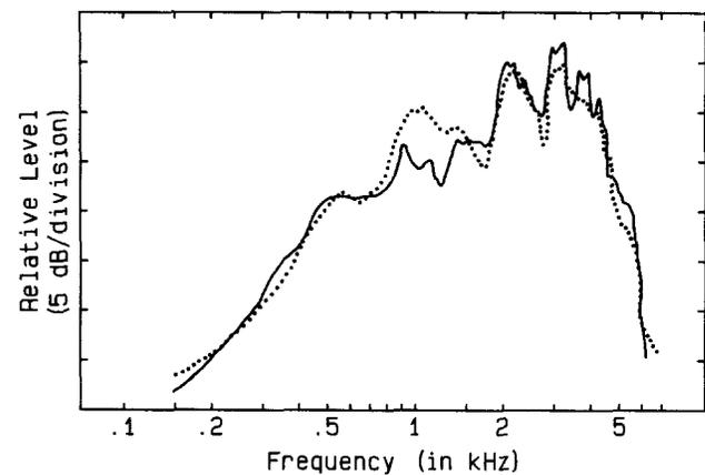
FIGURE 5. Damped (solid line) and undamped (dotted line) preferred listening levels for a typical wide bandwidth, normal speech input level condition. Shown are the Zwislocki coupler frequency responses for one of the three tested hearing aid pairs, averaged across 8 subjects.
