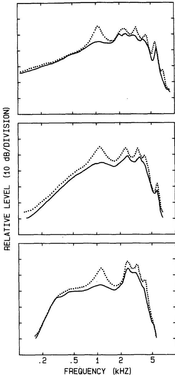
FIGURE 1. Damped (solid line) and undamped (dotted line) frequency responses for the three tested hearing aid pairs. Curves were measured in an HA-2 coupler with entrance via 25 mm of #13 tubing.
