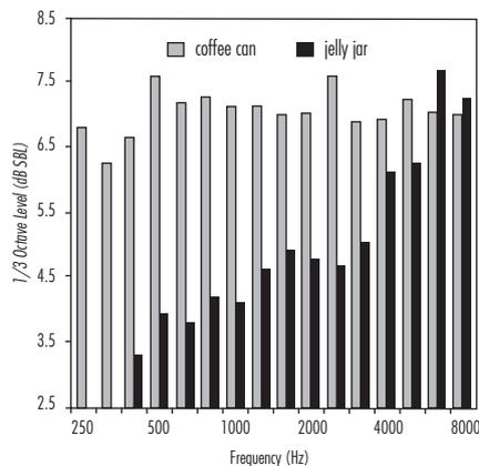
Figure 3. One-third octave band spectra for two noisemakers.
