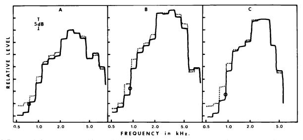
Figure 2. Frequency/gain curves, measured in one-third octave band levels, of the two tone control/earmold configurations used with each hearing aid from the second group of instruments. This group was defined as having low cutoff frequencies between 750 Hz and 1000 Hz. *Solid lines* depict the electronically modified condition. *Dotted lines* show the acoustically modified condition. *Open circles* indicate the derived low cutoff frequency for each instrument.
