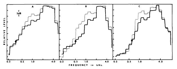
Figure 1. Frequency/gain curves, measured in one-third octave band levels, of the two tone control/earmold configurations used with each hearing aid from the first group of instruments. This group was defined as having low cutoff frequencies below 750 Hz. Solid lines depict the electronically modified condition. Dotted lines show the acoustically modified condition. Open circles indicate the derived low cutoff frequency for each instrument.
