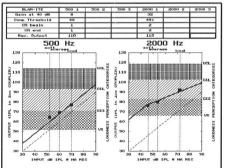
In this example, well-fitting I/O functions suggest a need for linear processing with about 8 dB gain in the low frequencies and input compression in the high frequencies with a compression threshold of 45 dB and compression ratio of 2.
